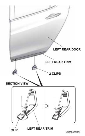
12. Using a rubber roller, apply firm pressure against the trim and roll from one end to the other. Apply firm pressure, especially at the ends.
