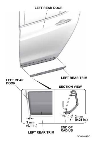
10. While applying light pressure against the trim, carefully remove the taped adhesive backings.
